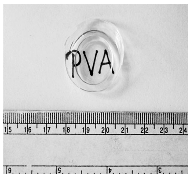
Fig. 1 A transparent PVA hydrogel synthesized by freeze-thawing
